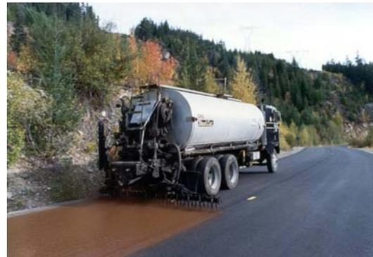
Highway rutting and subsequent deterioration of asphalt pavement are a continual problem in Whistler, British Columbia. Repair methods have varied from rehabilitative efforts to expensive full reconstruction. Recently, the municipality discovered the economic advantages of *reprofiling*, which uses hot-in-place recycling to return distressed pavement to like new condition, at the same time restoring a level profile from centerline to edge.
